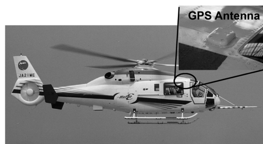
Fig. 1 JAXA's research helicopter and its GPS antenna installation.
